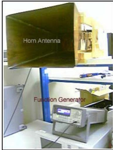
**Figure 3. Transmission hardware**
